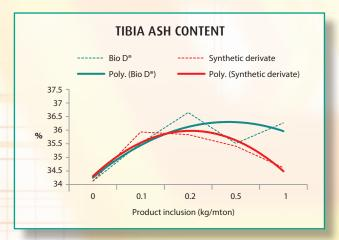
100 male broilers, Ross 708, per treatment were divided over 10 replicates. Two different sources of 25-OH D<sub>3</sub> were supplemented from day 0 till day 21 at different dosages. Tibia ash content was analysed on day 21.
